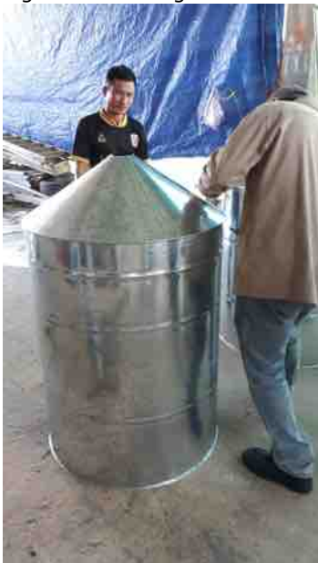
Figure 5. Building a hermetic metallic silo
